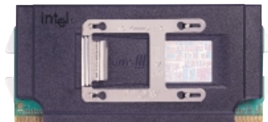
Example of an incorrectly installed retention clip
