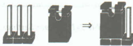
Figure 2 - 1 Jumper with Pins Shorted
