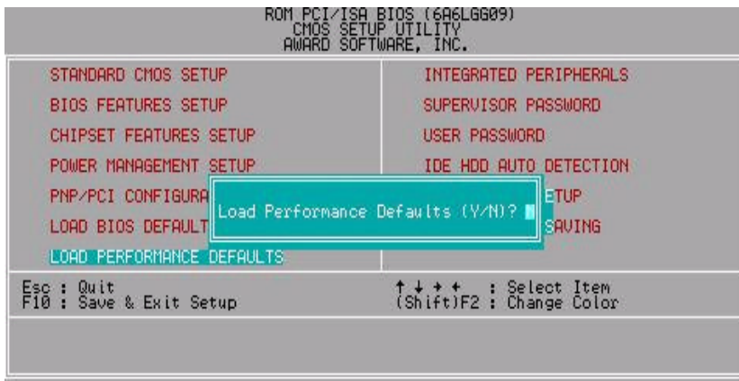
Figure 4.8: Load Performance Defaults
