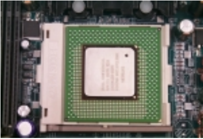
3. Align CPU and insert it
