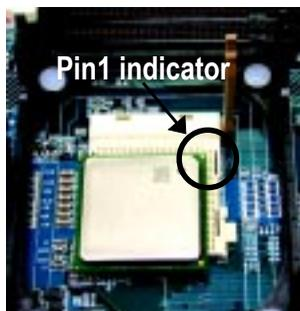
4. Locate Pin 1 in the socket and look for a (golden) cut edge on the CPU upper corner. Then insert the CPU into the socket.
