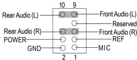
➤If you want to use "Front Audio" connector, you must remove 5-6, 9-10 Jumper. In order to utilize the front audio header, your chassis must have front audio connector. Also please make sure the pin assignment on the cable is the same as the pin assignment on the MB header. To find out if the chassis you are buying support front audio connector, please contact your dealer.
