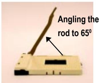
1. Angling the rod to 65-degree may feel a kind of tight, and then continue pull the rod to 90-degree when a noise "cough" made.
