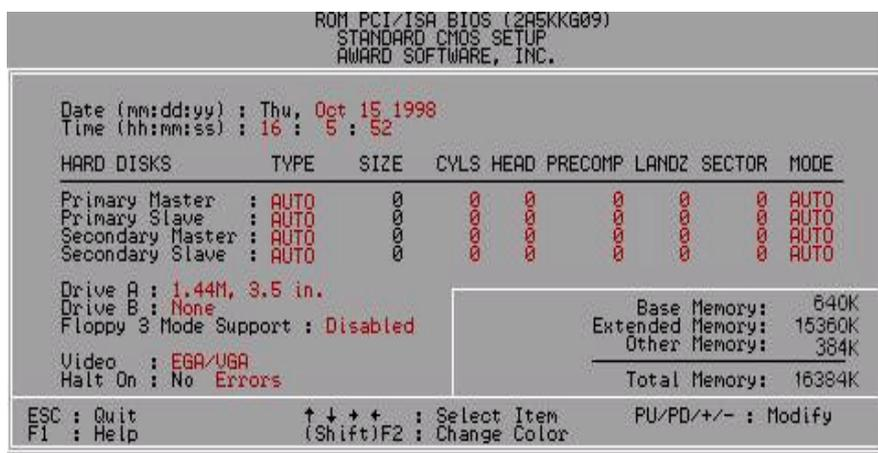
Figure 4.2: Standard CMOS Setup Menu
