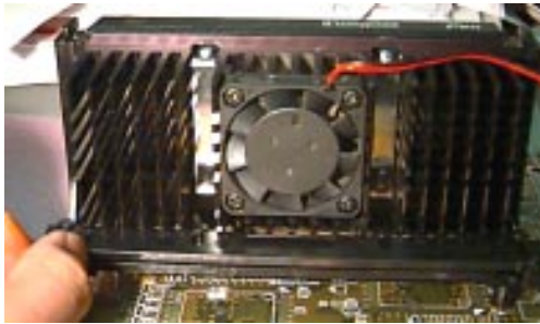
Heatsink Support Top Bar
