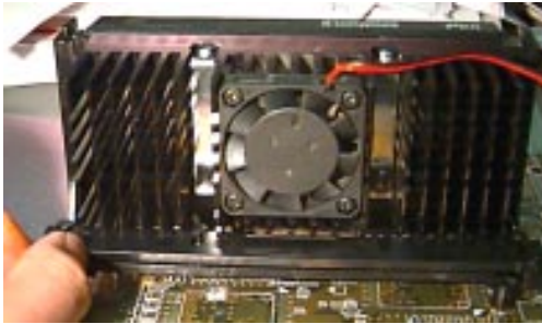
Heatsink Support Top Bar
