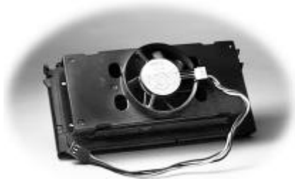
Pentium II Active (Boxed) CPU Shown with Power Connector for Fan
