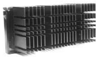
Pentium II Passive CPU Shown with Heat-sink
