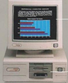
Integrated Video Graphics Controller makes the COMPAQ DESKPRO 286e ready to run VGA programs in addition to EGA and CGA
