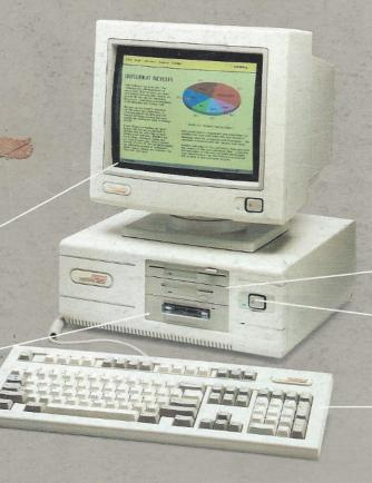
The system is the first to use the 16-MHz Intel 80386SX™ micro-processor and runs your software up to 60% faster than 10-MHz 286-based personal computers
