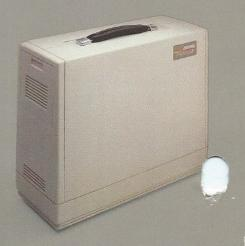
Based on the industry-standard 8-MHz 80286 microprocessor, the COMPAQ PORTABLE II Personal Computer is the ideal solution for people who need full-function desktop capabilities in a portable package. It delivers all the power and versatility most users need in a portable computer.
